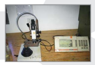
PLATING THICKNESS MEASURING MACHINE
