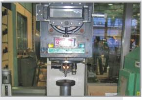
**VICKERS HARDNESS TESTER MACHINE**
